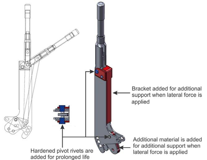
The RampTech E-Brake Lever recognizes a new standard for quality. We listened to users in the field and engineered a new and improved version of the Orscheln type lever originally used on the Tug MA. This new RampTech lever is designed for GSE and the ramp and will last longer than the original. Added strength was developed for enhanced improvement and performance.
